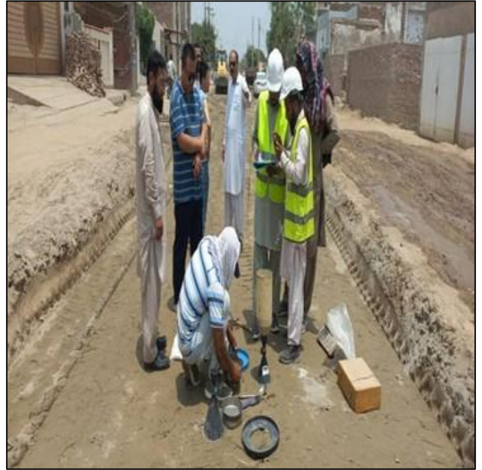
Picture 14: L-2.5 42" dia sand FDT test
